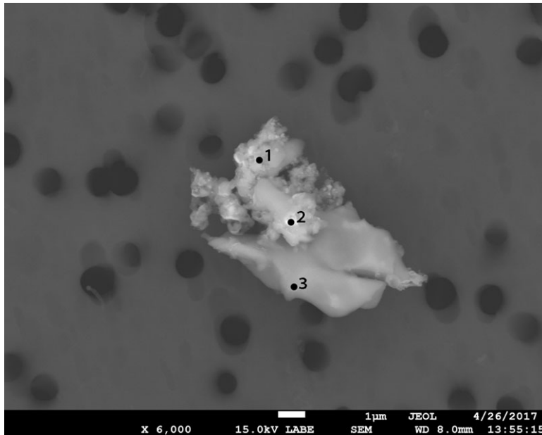
SEM Photo of sample L2101 A1 with labeled EDS testing locations.
