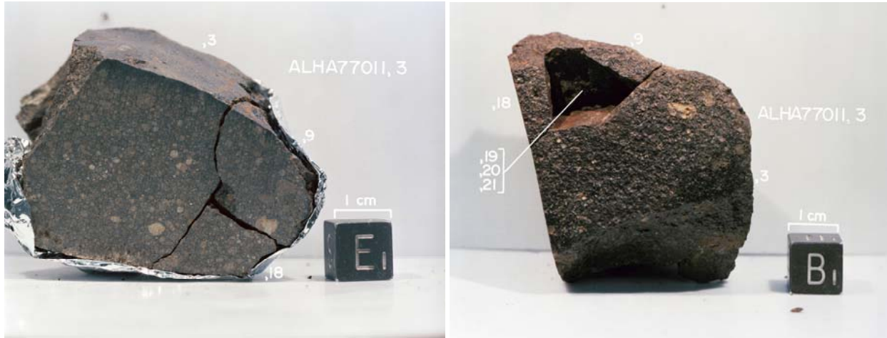
Figure 7: Laboratory photos of ALH A77011 illustrating the fusion crusted exterior (right; NASA photo S81-32616) and the chondrules, matrix and inclusions in the interior (left; NASA photo S81-32618).
