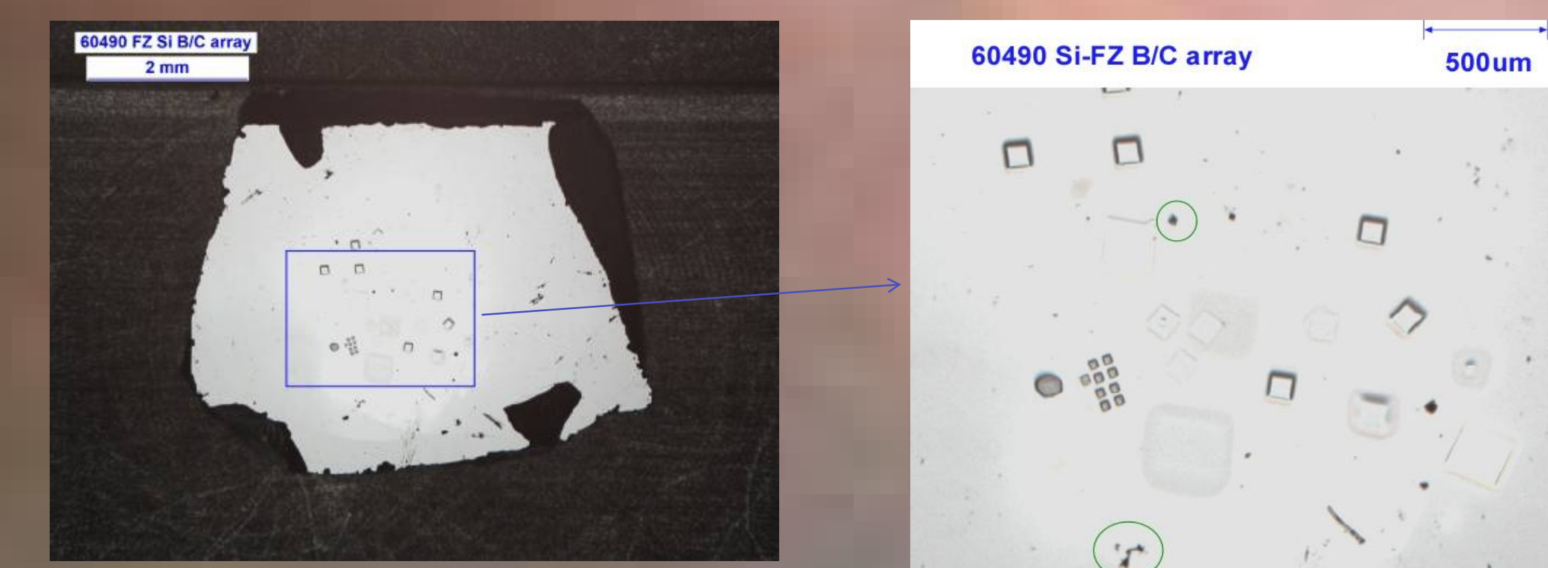
After allocation: Images were taken after 80 hours of aqua regia cleaning plus RCA cleaning. No white ovals can be seen.
