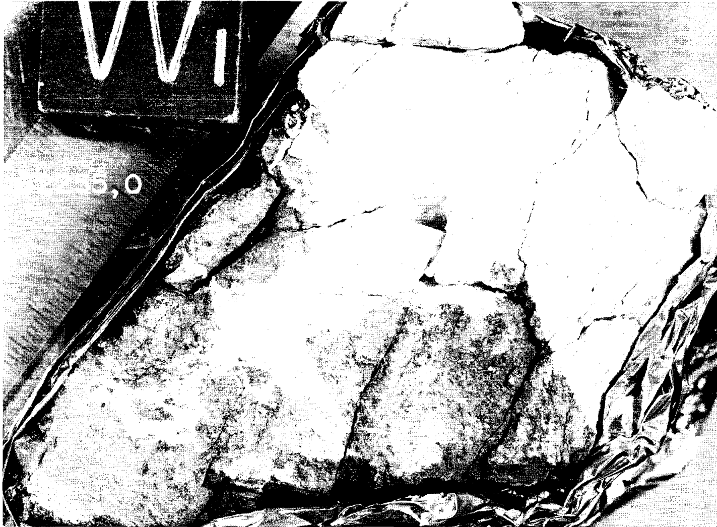
Figure 3. Sawn surface of 62255, showing relation of anorthosite (white) to dark aphanitic material. (NASA S-75-33052)
