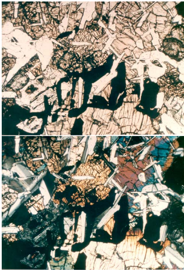
Figure 3: Photomicrographs of thin section of 10044 (top is plane polarized light, bottom is with crossed-polarizers). Field of view is 2.5 mm. NASA S70-49983 and 49984.
