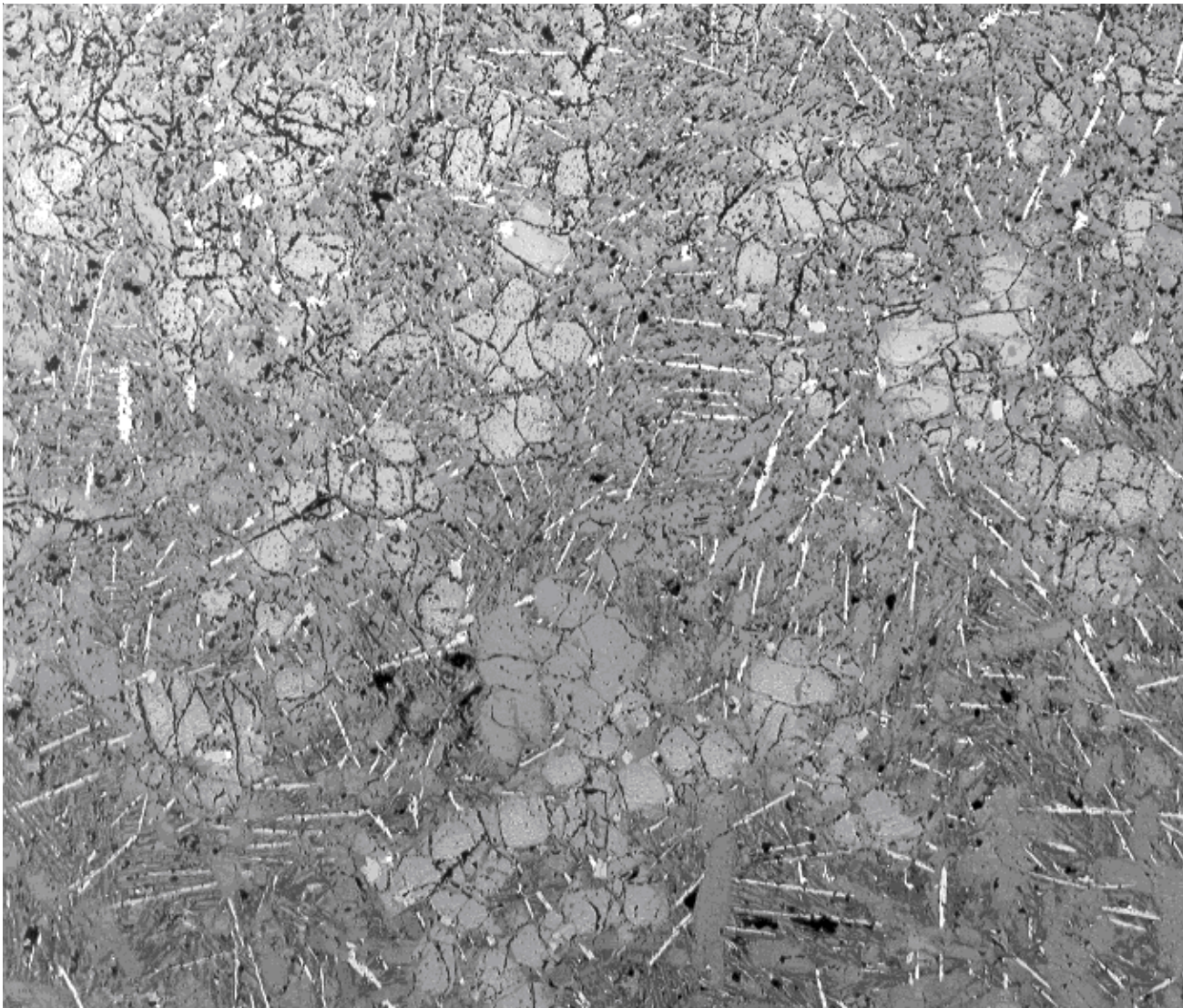
Figure 2: Reflected light photo of thin section 12022,10 showing alignment of ilmenite, clumps of pyroxene phenocrysts in fine-grained variolitic groundmass. Field of view 1 cm. NASA photo # S70-24742.
