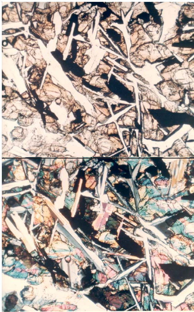
Figure 3: Photomicrographs of thin section 12051,62 (plane-polarized, crossed-nicols). Field of view 2.6 mm. NASA # S7049833-834.
