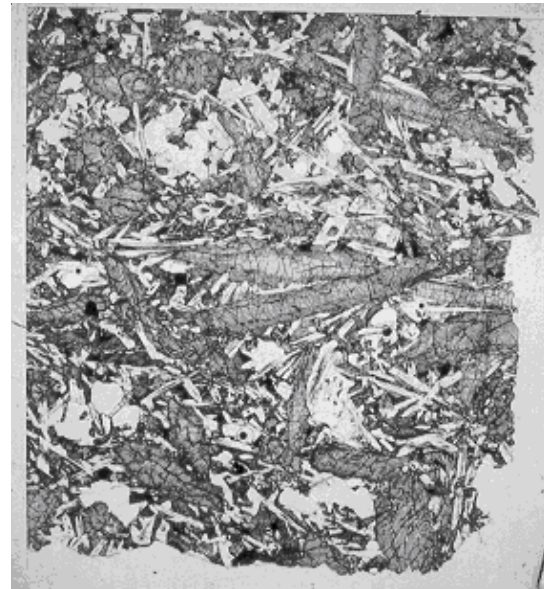
Figure 3: Low magnification photo of microscope slide showing elongate pyroxene crystals and radiating plagioclase laths in 15058,128. Scale is about 1 cm.
