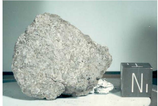
Figure 1b: Photo of 15085 showing basaltic texture. Cube is 1 inch. NASA S71-43088.
