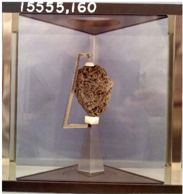
Figure 22: Display case with 15555,160. Case is made from optical glass and filled with dry nitrogen.
