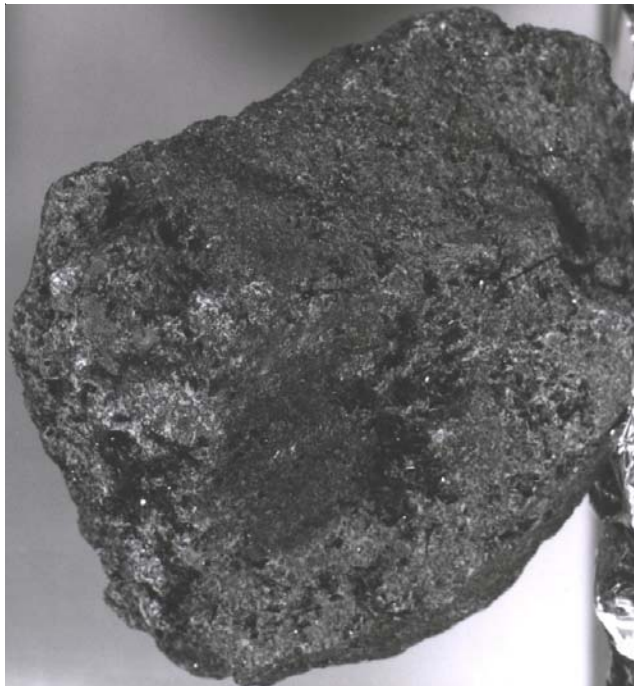
Figure 2: Photo of bottom, freshly broken surface of 70185 showing numerous vugs. NASA S73-17312. Sample is about 7 cm across.
