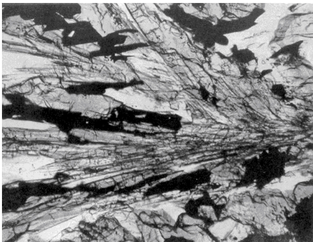
Figure 5: Thin section photo of 71055,68 showing unusual subvariolic structure (by Neal and Taylor 1993). Field of view is 2.5 mm.
