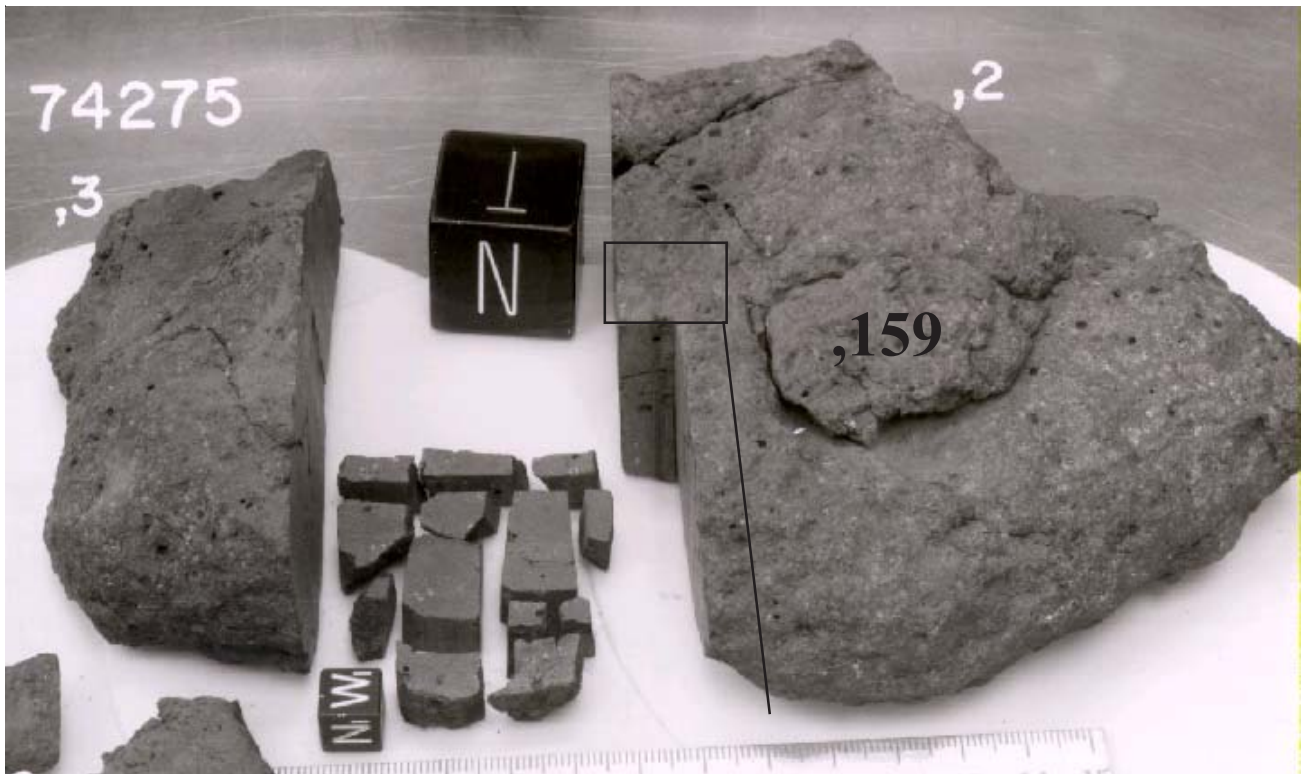
Figure 19: First partial slab cut from 74275. Position of first column and second slab indicated. NASA# 73-28789. Nice illustration of our 1 cm cube as well as our 1 inch cube!
