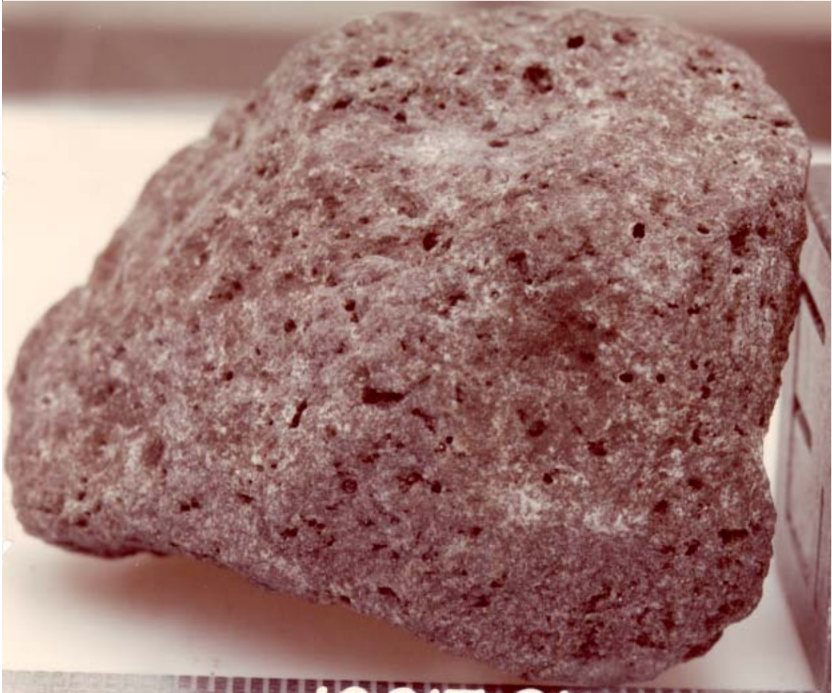
Figure 1: Close-up photo of dusted surface of 10017,81 N1 face. Sample is 4 cm across. NASA #76-25451.
