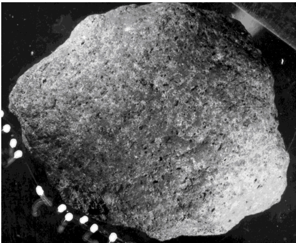
Figure 3: Original photo taken in F-201 of “flatter” side of 10017,0 showing numerous, well-developed micrometeorite craters. This side was eventually determined to be the most recent top surface, because it had abundant short-lived radionuclides (see text). NASA S69-47560. Sample is 16 cm long.
