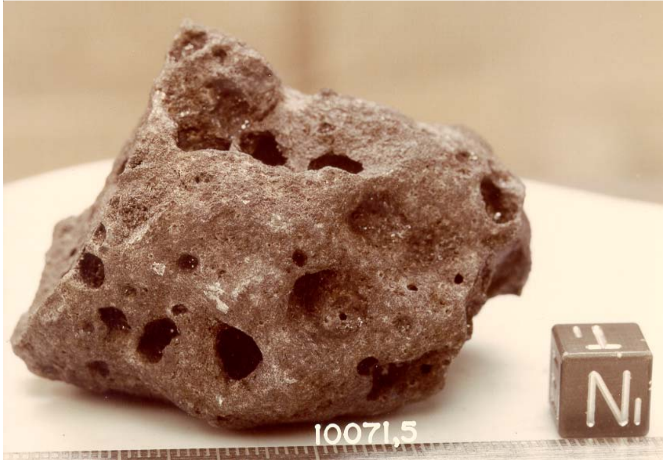
Figure 1: Photo of 10071,5 illustrating large vesicles and smooth surface, rounded by micrometeorite bombardment. NASA S76-22608. Cube is 1 cm.
