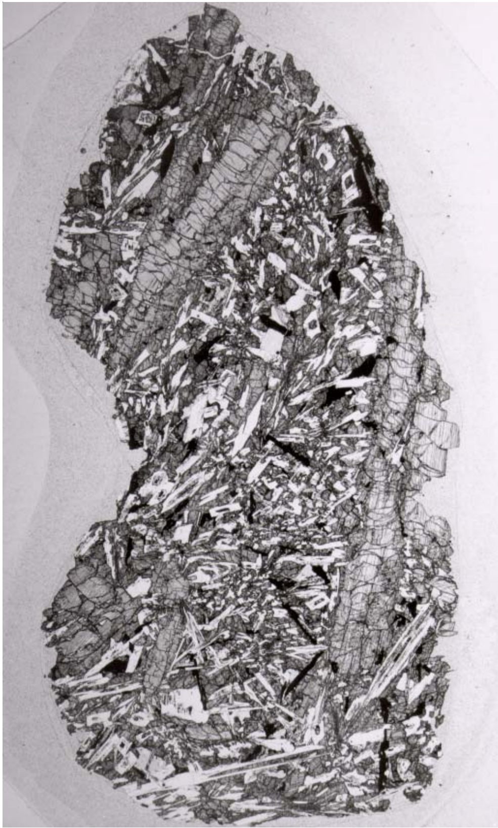
Figure 2: Photomicrograph of thin section of 12021,3 showing elongate and sector-zoned pyroxene. Field of view is 3 cm. NASA # S70-25401.
