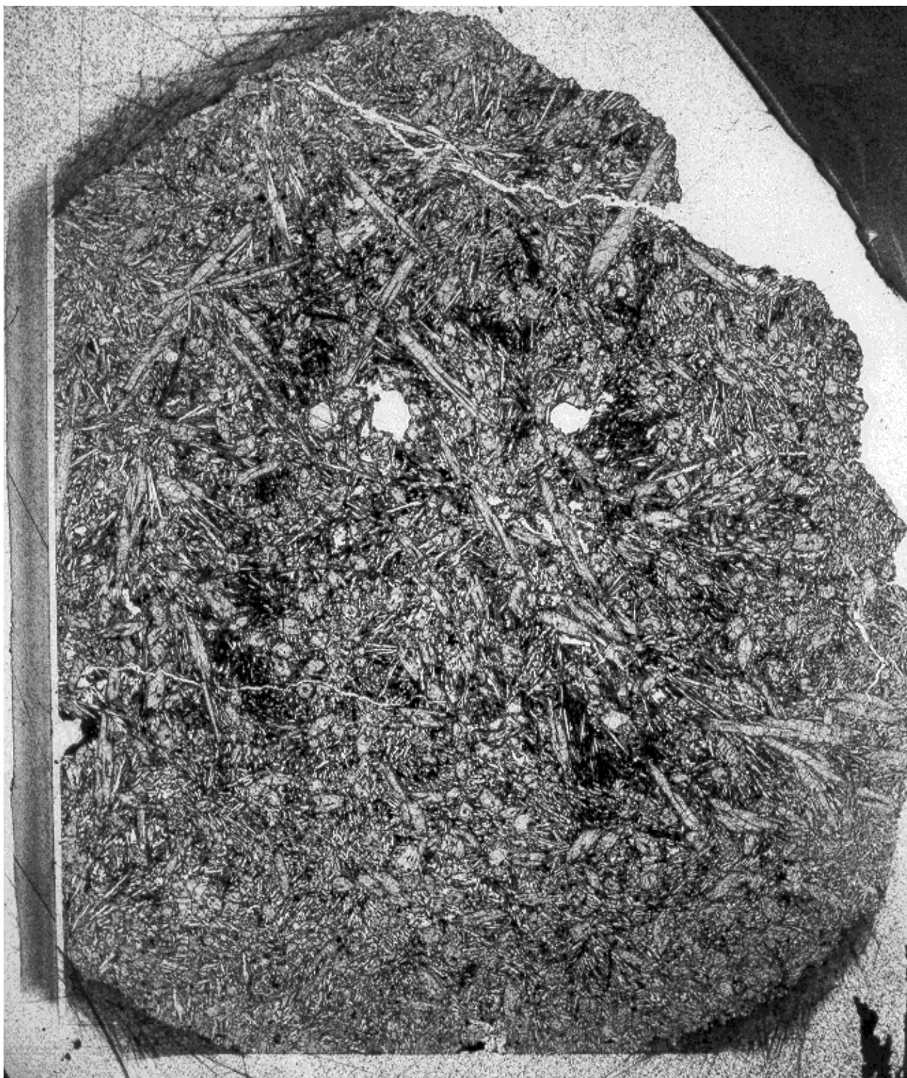
Figure 2: Transmitted light photomicrograph of thin section 12053,75 showing long, hollow pyroxene phenocrysts in variolitic groundmass. Section is about 3 cm long. NASA #S70-36473.
