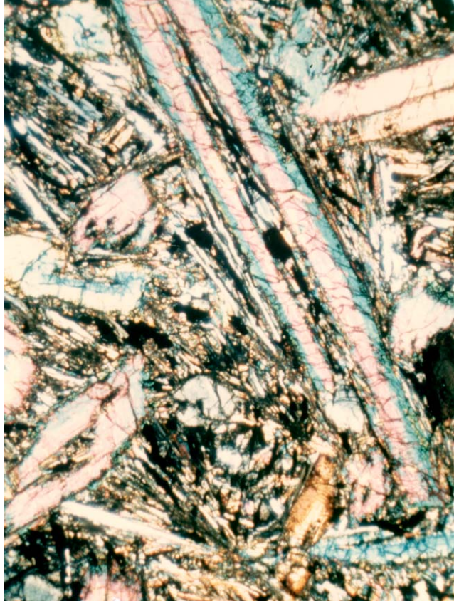
Figure 3: Transmitted-light and crossed-nicols of thin sections 12053,75 (top) and 12053,91 (bottom) showing chemically zoned, hollow, pyroxene phenocrysts (elongate and in cross section) set in variolitic groundmass.
