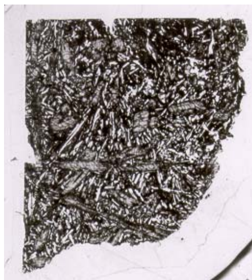
Figure 2b: Transmitted light photomicrograph of 12052,8 showing random pyroxene and plagioclase. Scale 1 cm. NASA #S70-51003.
