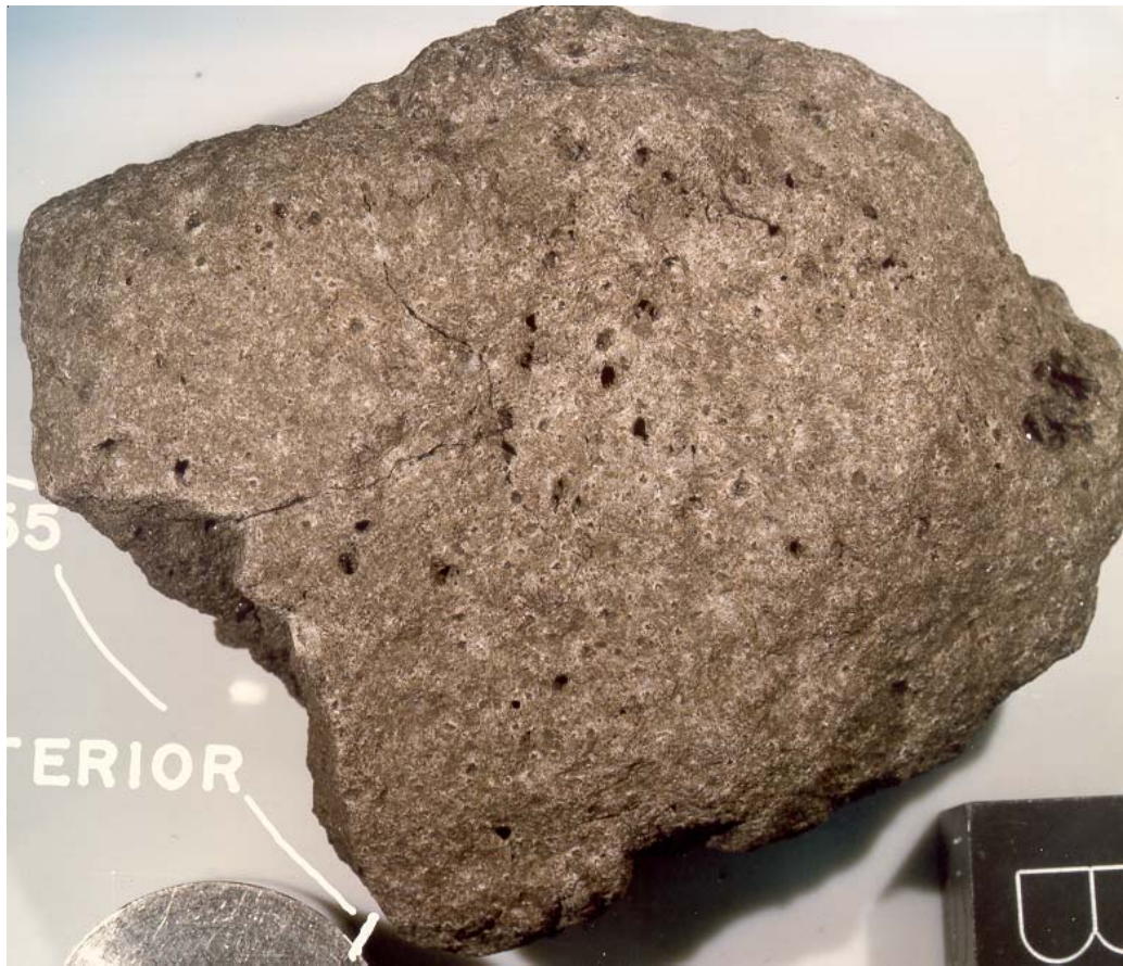
Figure 6: Large portion of 12055,0 showing zap pitted surface with vesicles. Cube is 1 inch. NASA #S86-38615.
