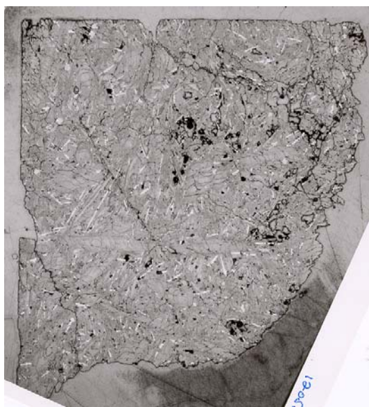
Figure 2a: Reflected light photomicrograph of 12052,8 showing porosity and random ilmenite. Scale is 1 cm.
