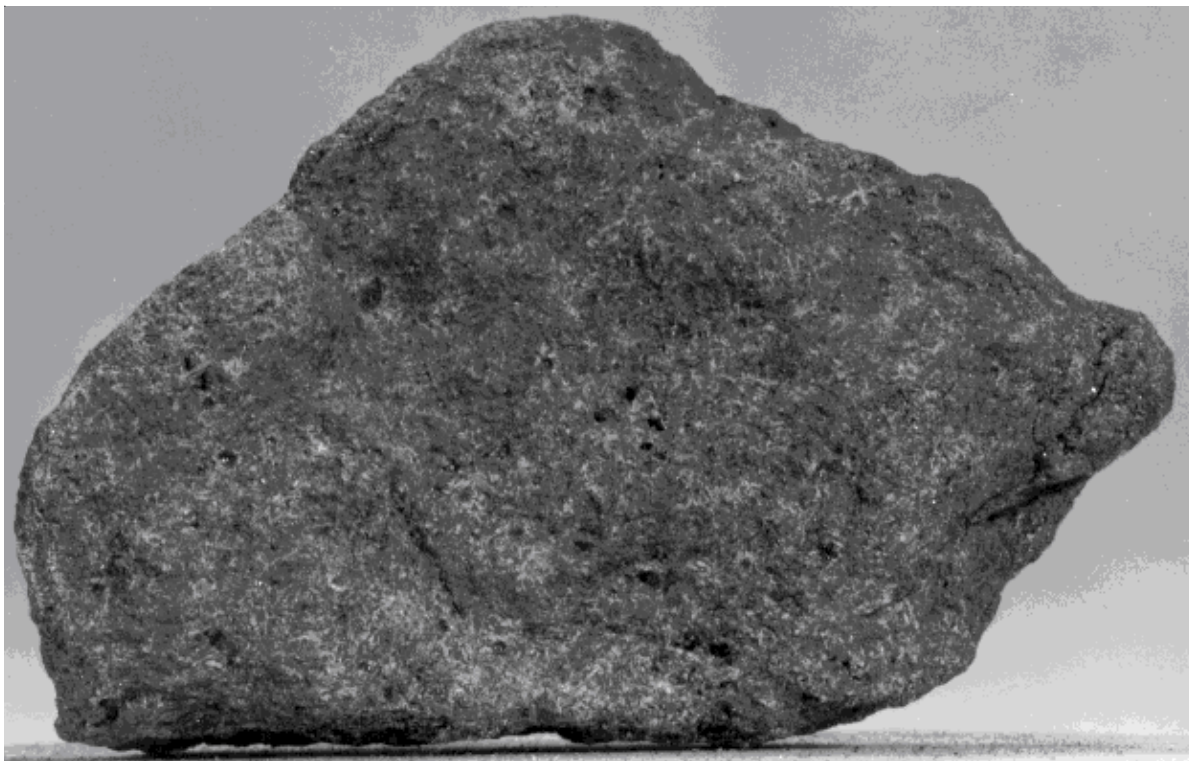
Figure 2: Photo of rounded top of 12056 showing zap pits. Rock is about 7 cm across. NASA # S70-19062.
