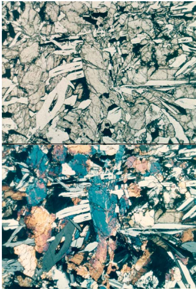
Figure 4: Photomicrographs of thin section 12063,19 (plane-polarized light; crossed-nicols). NASA # S70-49543-49544. Scale 2.6 mm.
