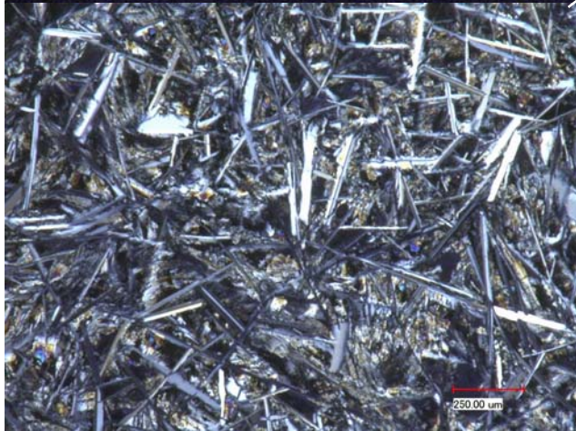
Figure 6b: Photomicrographs of thin section 14077,2 by C Meyer at 50 x and 150 x (crossed polarizers).
