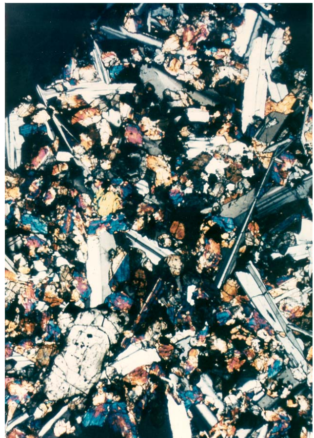
Figure 3: Thin section photos of 15556 (same area as figure 2). a) plane polarized light, b) crossed polarizers. NASA S71-51762-3. Scale about 2 mm.
