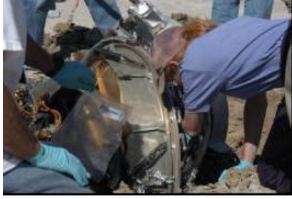
Figure 2. The as-landed condition of the spacecraft before securing the unfired ordnance and the half buried science payload canister. Team members are removing loose collectors.
