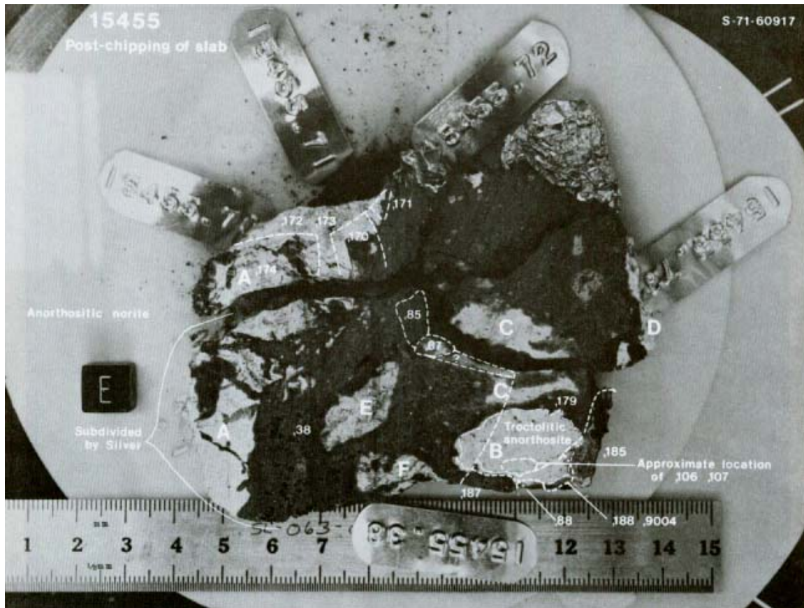
Figure 2. Chipping slab cut from 15455 showing lithologies and split numbering. S-71-60917
