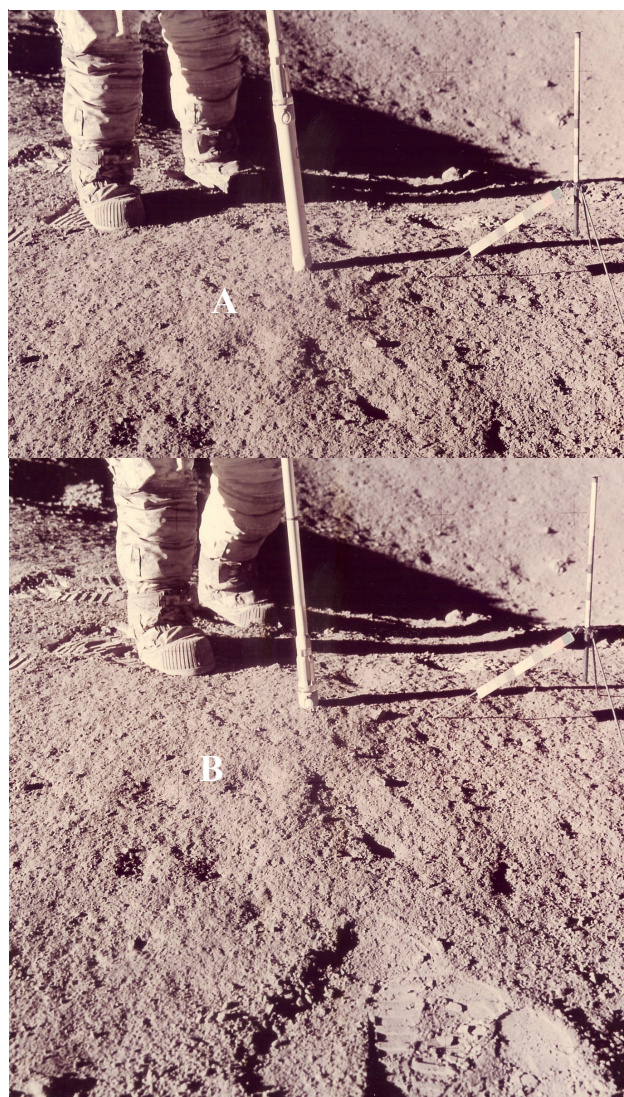
Figure 9: Doube drive tube 15008/7 during insertion into soft rim of small crater.
