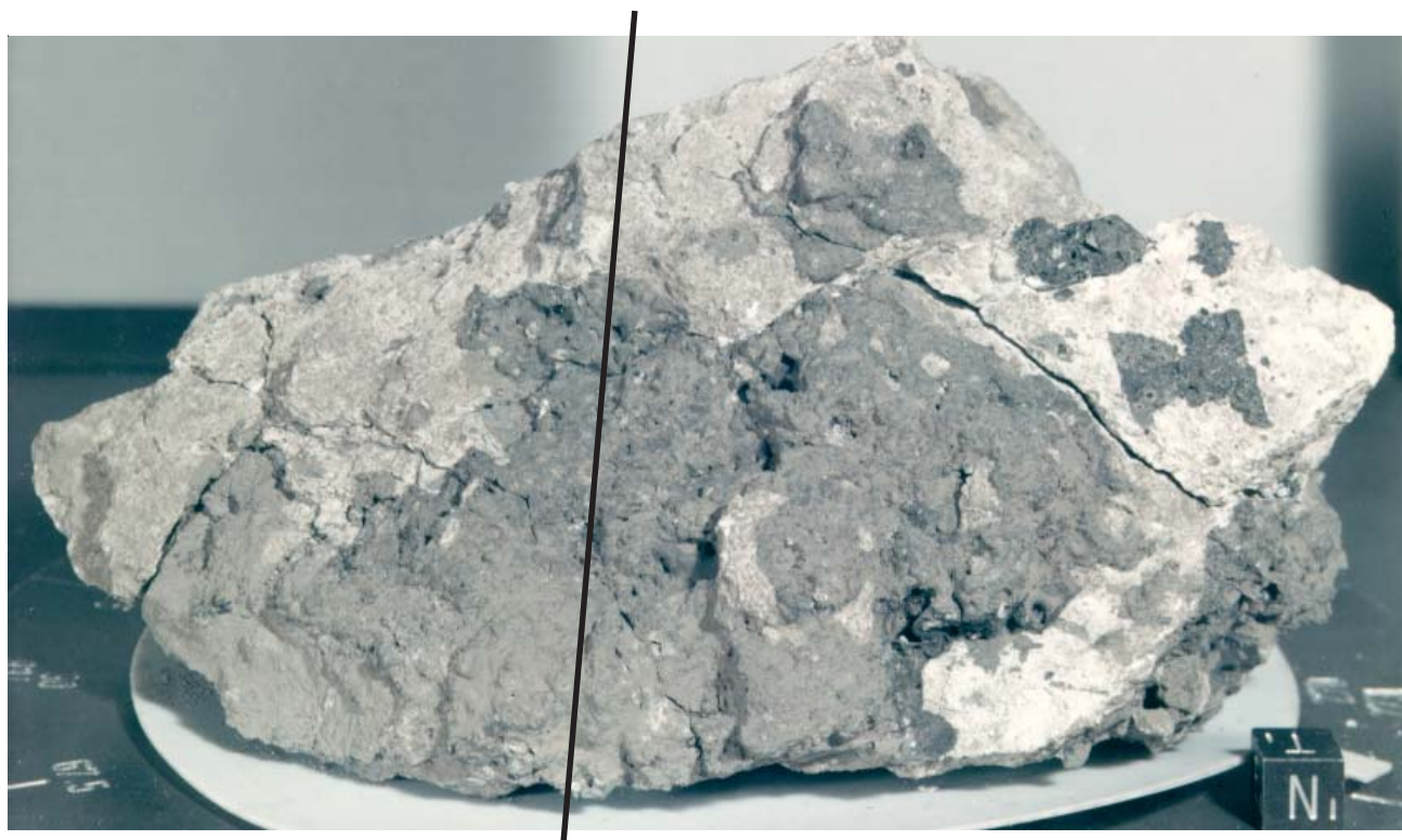
Figure 1: Photo of 62255 showing glass splash on anorthosite. Cube is 1 cm. NASA S # S72-38309.
