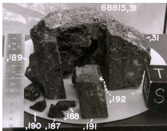
Figure 16: Group photo of saw cuts to produce column 68815,192 and ,191. NASA # S74-27981.
