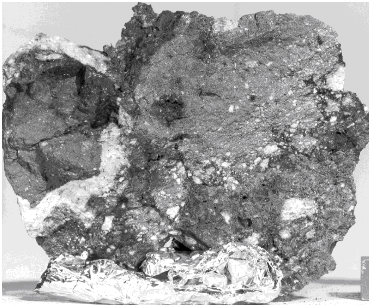
Figure 3: Photo of fresh-broken side (B1) of 69935. NASA S72-44459. Edge of cube is 1 cm. Note the white clast. Ignore the Al-foil.
