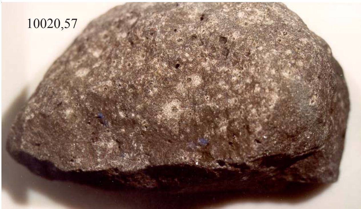
Figure 7: Photo of 10020,57 showing micrometeorite craters (zap pits). Sample is 6 cm long. NASA S84-35315.
