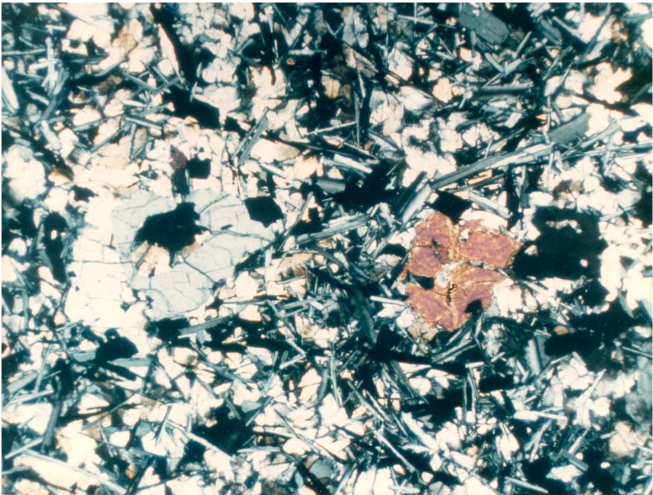
Figure 2: Photomicrograph of 10020,40 showing apparent xenocrysts in basaltic texture. Field of view 2.5 mm across. NASA S70-49470.
