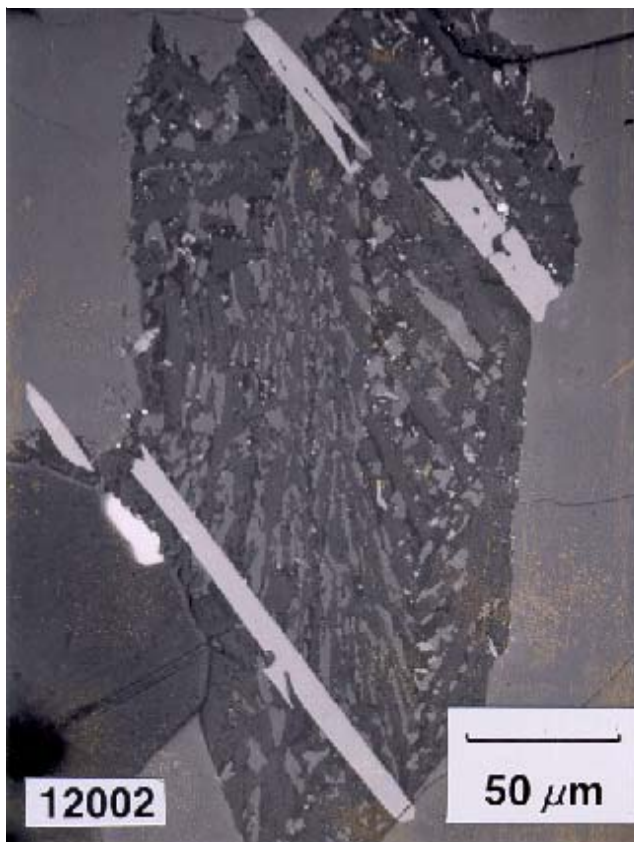
Figure 5: "Melt inclusion" in pyroxene phenocryst (now crystallized).
