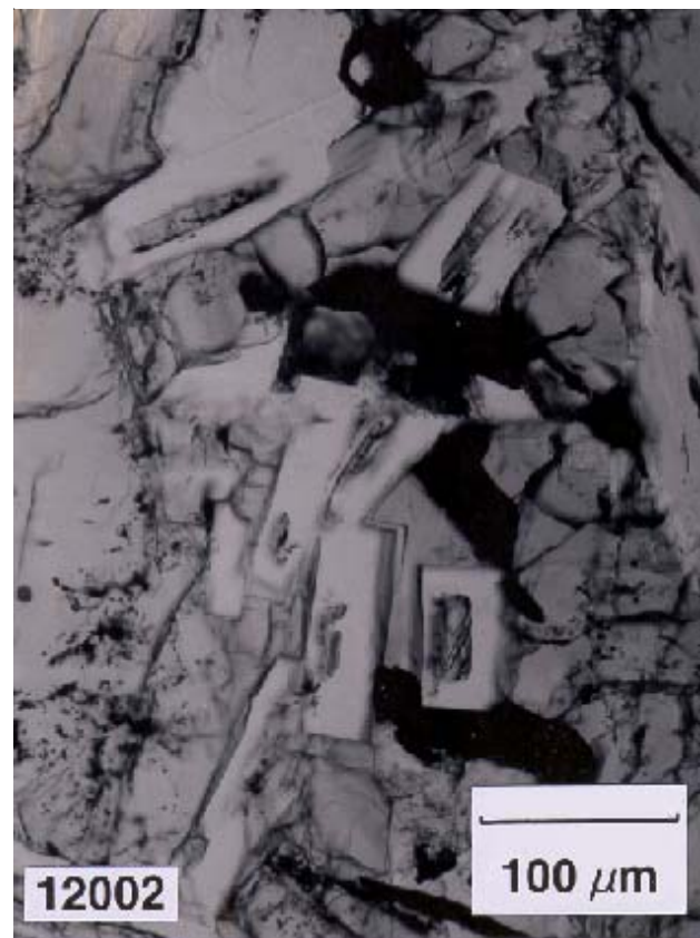
Figure 6: Hollow plagioclase "straws" in cross section in 12002.
