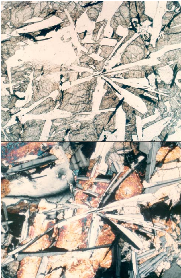
Figure 3b: Photomicrographs of thin section 12038,2 (top = plane-polarized light; bottom = crossed-nicols). Scale 2.2 mm. NASA S70-49437-438.
