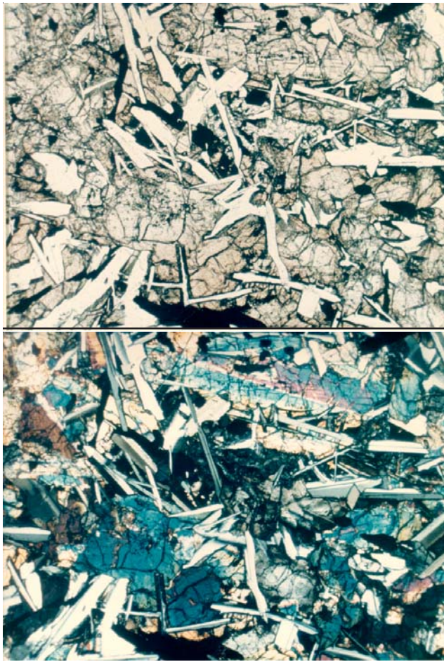
Figure 3: Photomicrographs of thin section 12062,11 (plane-polarized, crossed-nicols). Field of view is 2.6 mm.
