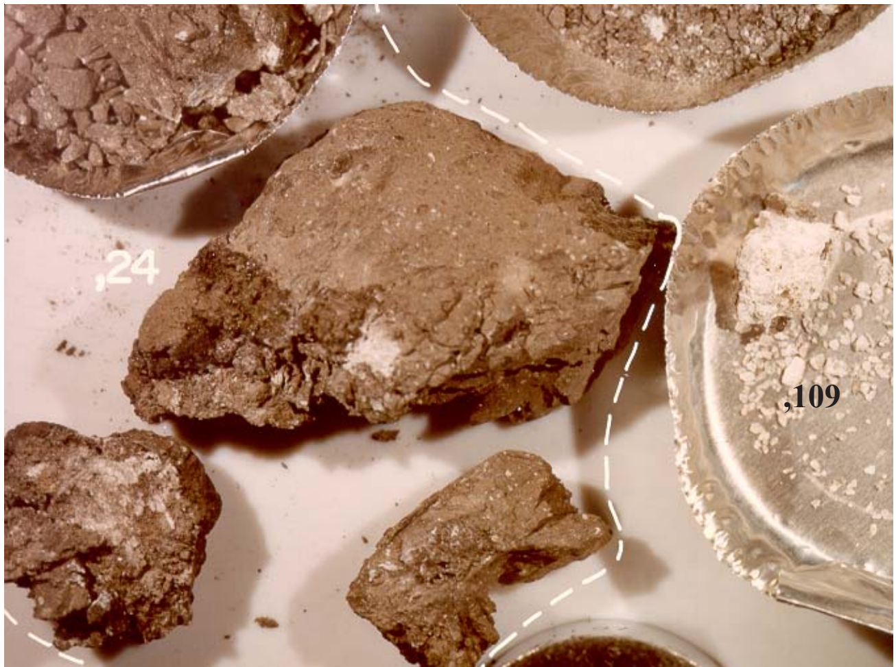
Figure 10: Photo of 14047 pieces after extraction of large white clast in 1980. Largest piece, 24 is 5 cm: white piece ,109 is about 1 cm. NASA S80-38169.
