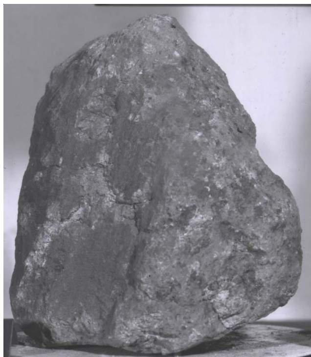
Figure 1: Photo of 14301 showing side with striations in packed dirt. NASA S71-32473. Sample is 10 cm.
