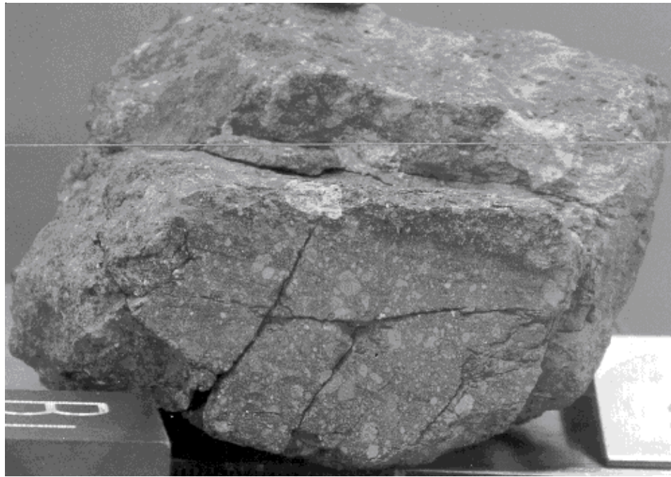
Figure 16: 14318 after first saw cut with wire saw positioned for second cut to make slab. Sample is about 10 cm across. NASA S71-38662.
