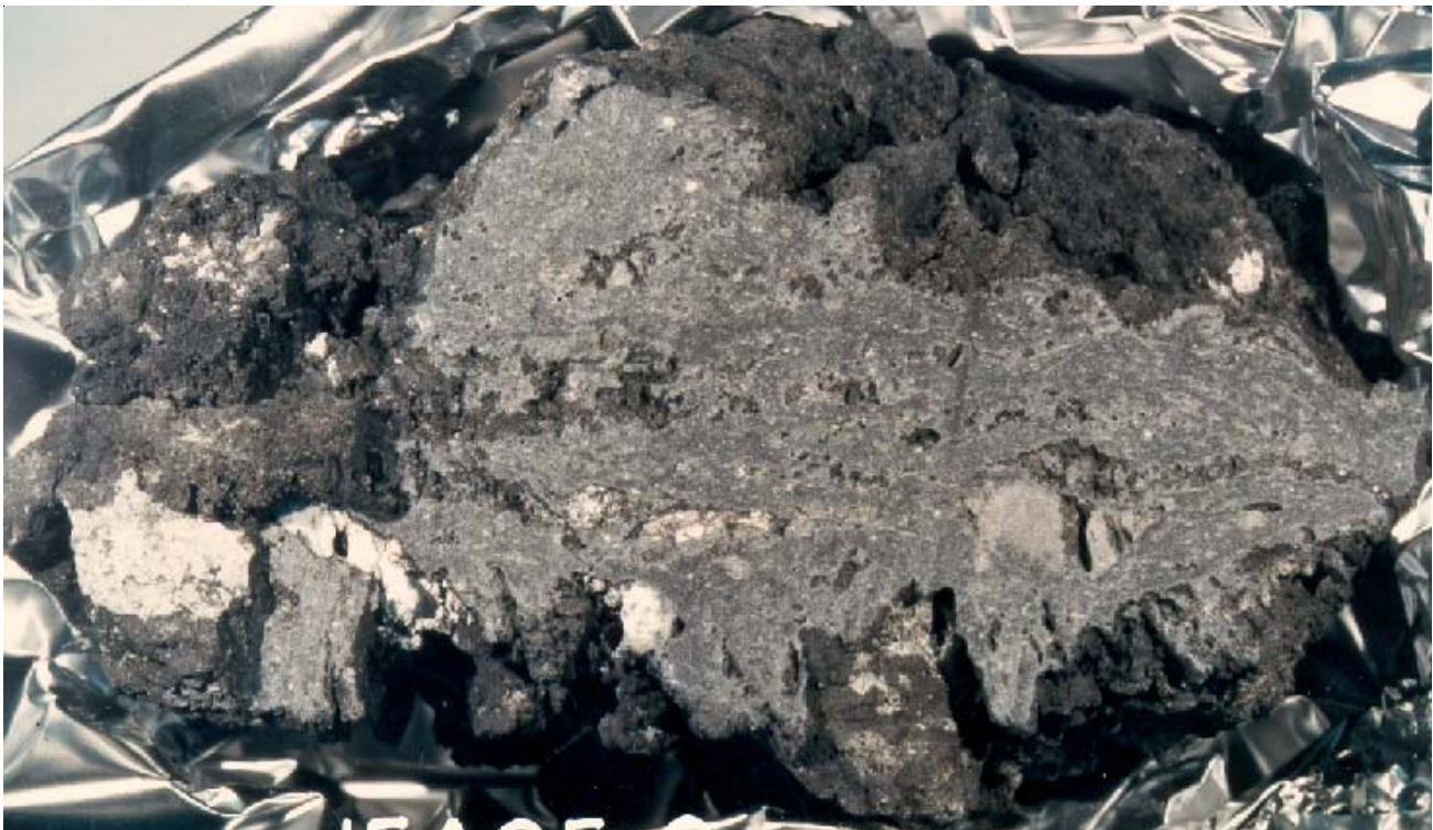
Figure 5: Photo of sawn surface of 15405,0 showing clasts and 'flow-banding' in matrix. S85-38199. Sample is about ~ 9 cm long and prominent white clast is ~ 0.9 cm long.
