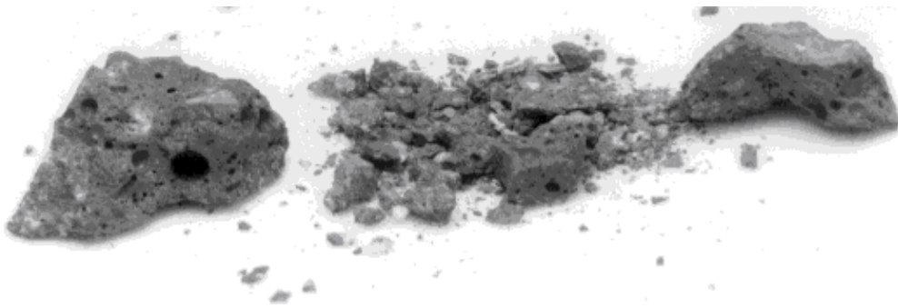
Figure 10: Photo of 15418,1 illustrating vesicularity. Large piece is 2 cm across. NASA S72-32321.
