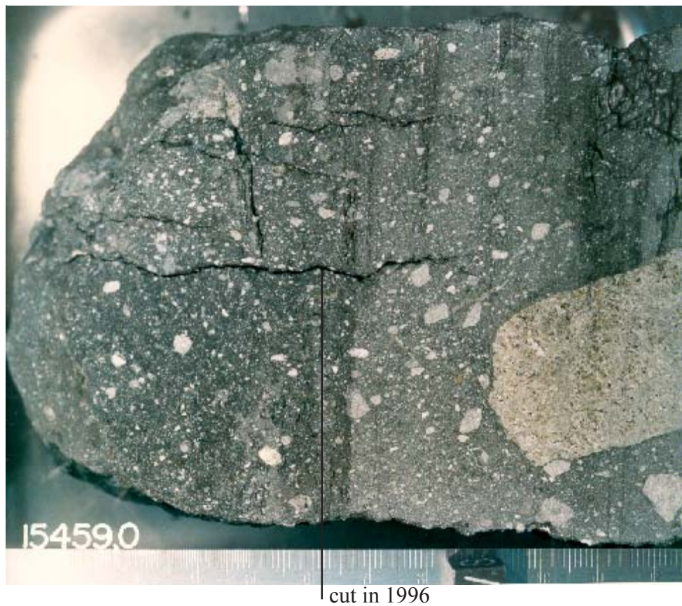
Figure 2: Photo of sawn surface of 15459,0 after slab removed in 1985. Location of right angle cut in 1996 is shown. Scale is in cm. Large clast is picritic basalt. NASA# S85-42240.
