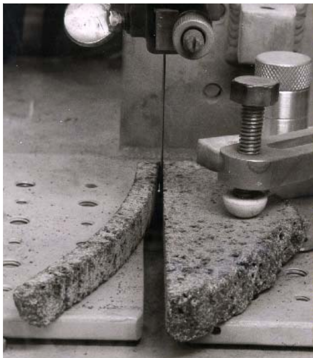
Figure 21: Sawing slab. Photo # S71-57094.
