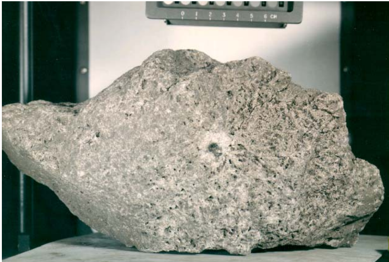
Figure 1: Photo of S1 surface of 15555, illustrating large micrometeorite crater (zap pit) and vuggy nature of rock. NASA S71-43954. Scale is in cm.
