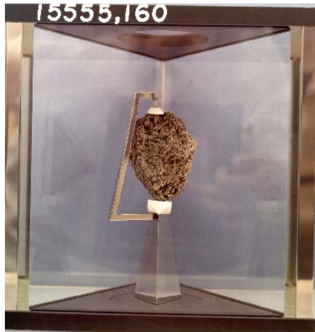
Figure 23: Display case with 15555,160. Case is made from optical glass and filled with dry nitrogen.
