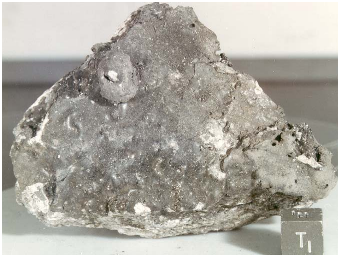
Figure 1: Photo of glass coated side of 60639. Cube is 1 cm. NASA S72-43469.
