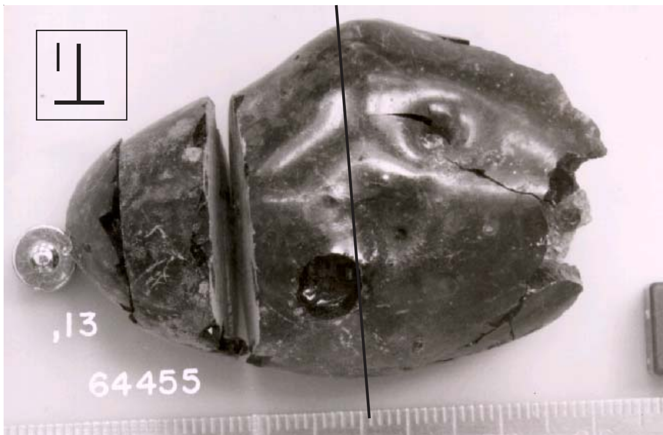
Figure 14: Photo of the T1 surface (lunar bottom) of 64455 after cutting first slab A. The approximate location of the second slab is indicated by the line. The scale is in mm and the cube is 1 cm. There are no zap pits on this surface as it was below the soil line. Photo # S72-53870.
