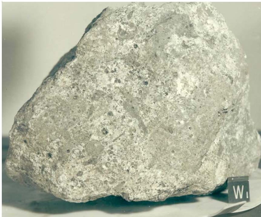
Figure 2: Top surface of 66055 showing numerous zap pits. Cube is 1 cm. S72-39298.
