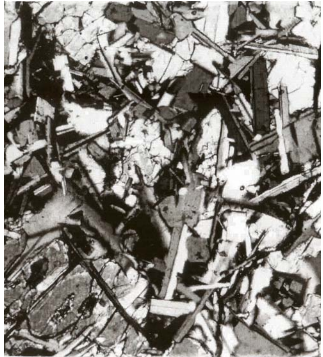
Figure 2a: Thin section photo (crossed-nicols) of 67747,1,
