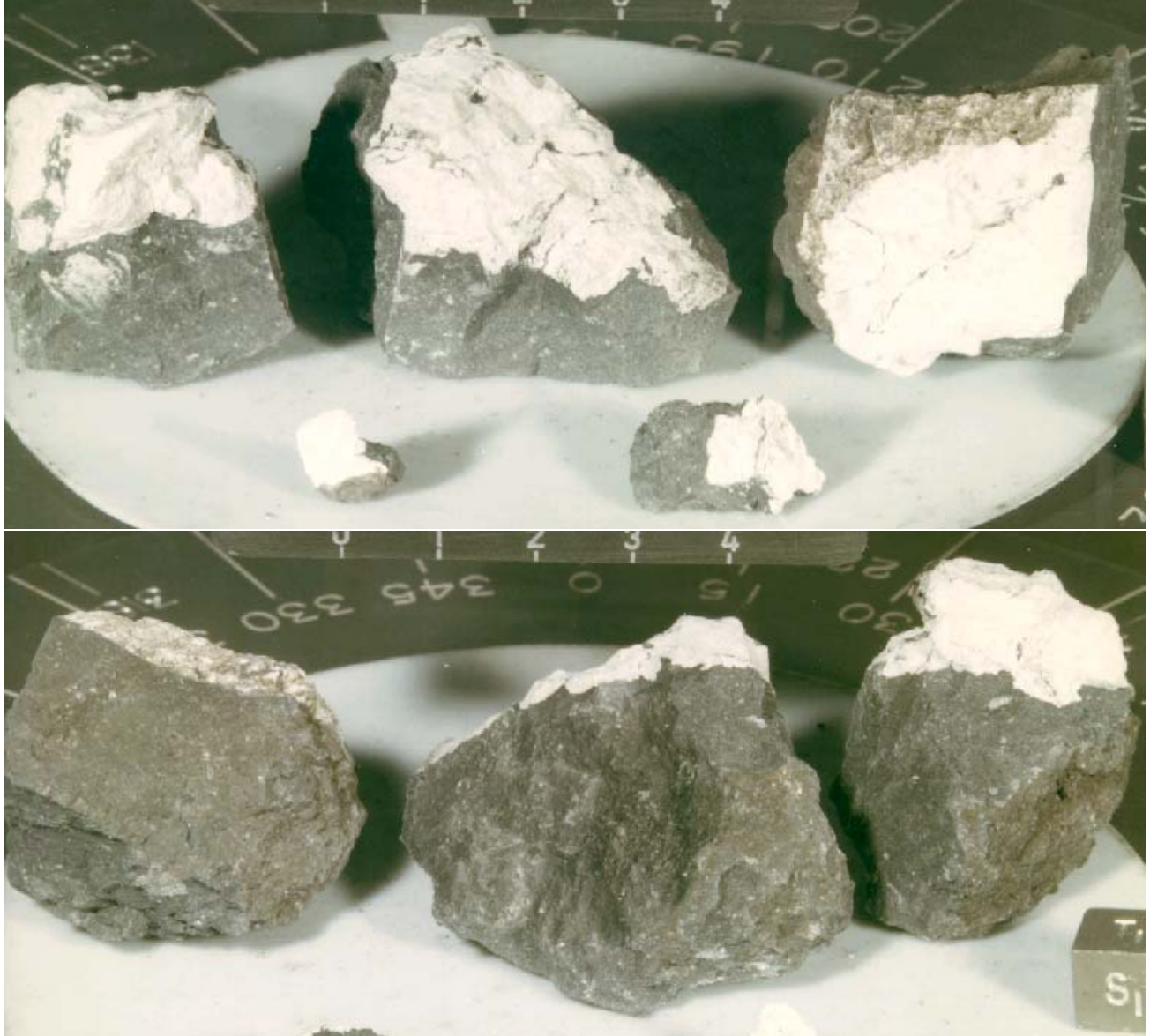
Figure 1: Front and back photos of 77075. Scale and cube are 1 cm. NASA# S73-17186 and S73-17185. These pieces were found to fit together (see figures 14, 15 and 16)..
