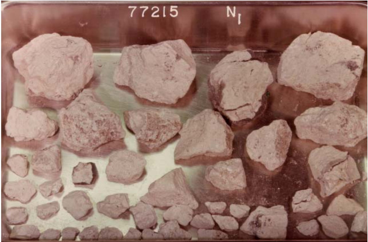
Figure 1: Tray full of pieces of 77215. Some pieces are covered with “off-white” patina including obvious zap pits. NASA photo # S73-17779.
