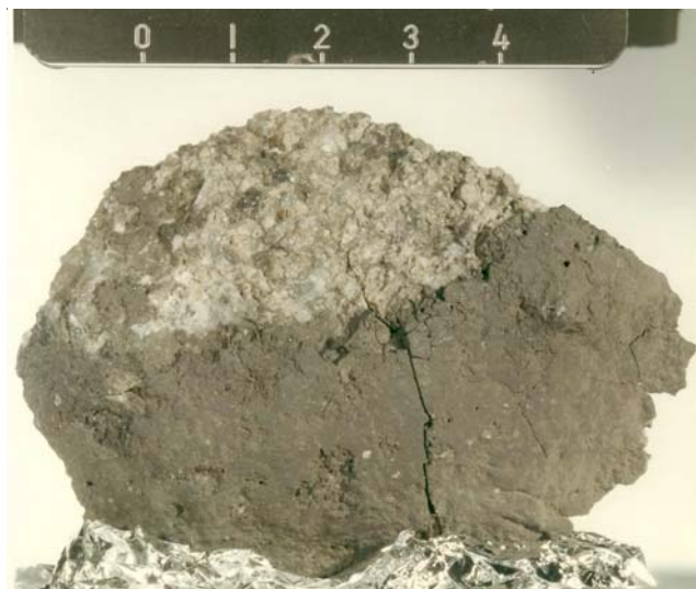
Figure 22: Reverse side of 78236 - see also figure 3. The whole bouldr was covered with this thick brown glass coating.
