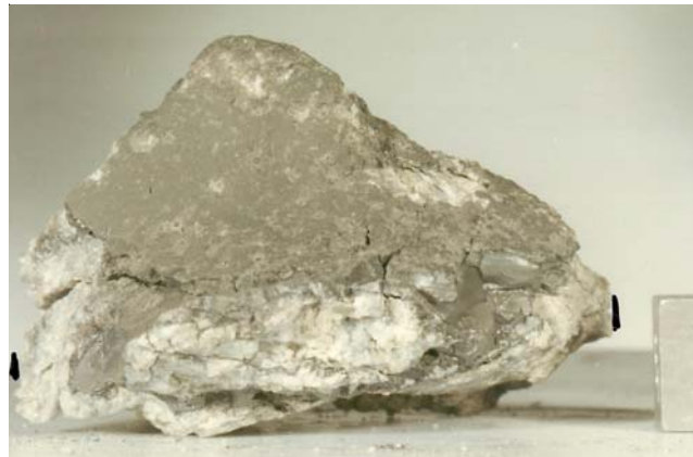
Figure 5: The outer surface of each piece was coated with 1/4 inch of brown glass. This is the reverse side of 78238 in figure 4. S73-15463.
