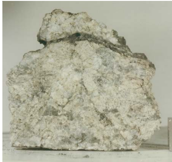
Figure 4: Photo of 78238 showing glass vein. Side of 1 cm cube is showing at right. NASA S73-15461
