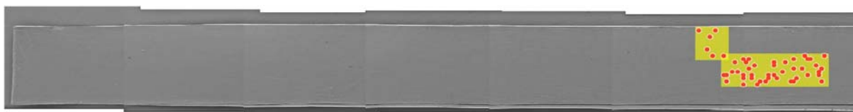
Figure 3a: Craters on Al foils 037N (left half). The yellow-shaded areas were systematically scanned for the presence of craters with sizes > \sim 200 nm. The locations of craters are indicated by red dots. Dito in Figs. 3b-d. The coordinates of the craters and of the corners of scanned fields are given in Appendix A.
