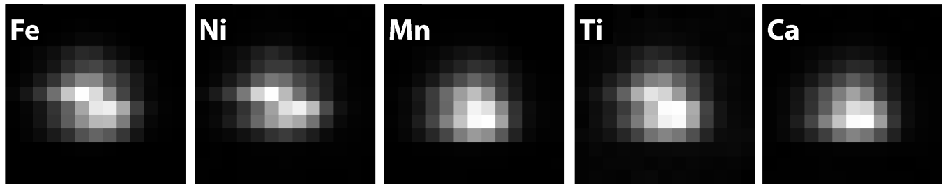
Fig 17. Fluorescence maps of 13 \times 13 pixel area ( 1 \mu\text{m}/\text{pixel} ) of terminal particle, C2092,82, a) Fe K\alpha , b) Ni K\alpha , c) Mn K\alpha , d) Ti K\alpha , e) Ca K\alpha .
