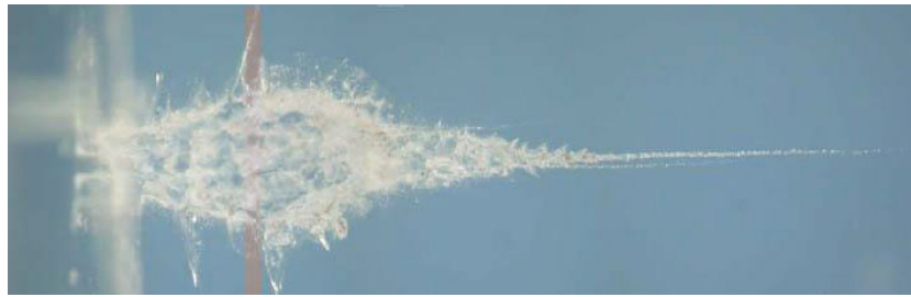
Fig. 1. Track 41. This is a Type B “turnip” shaped track of length \sim 4 mm and the impact was from the left of the image moving right. It was removed from the cometary collector cell 44. (See Burchell et al. 2008 for a discussion of track nomenclature and the distribution of tracks in the collector tray. An extended discussion of the characteristics of Type B tracks is given in Trigo-Rodríguez et al. 2008.). Our slice was cut 0.8 mm in (gray vertical rectangle) from the track entrance. Track image courtesy of NASA JSC.
