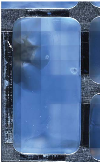
Fig. 1. Optical image of aerogel cell C2004 from NASA-Johnson Space Center (JSC) level 2 photo documentation using reflected light. The cell is 4 cm high and 2 cm wide. Track 44 is the large impact feature in the upper left. The impacting particle struck the edge of the tray frame (white arrow) before bouncing into the aerogel.
